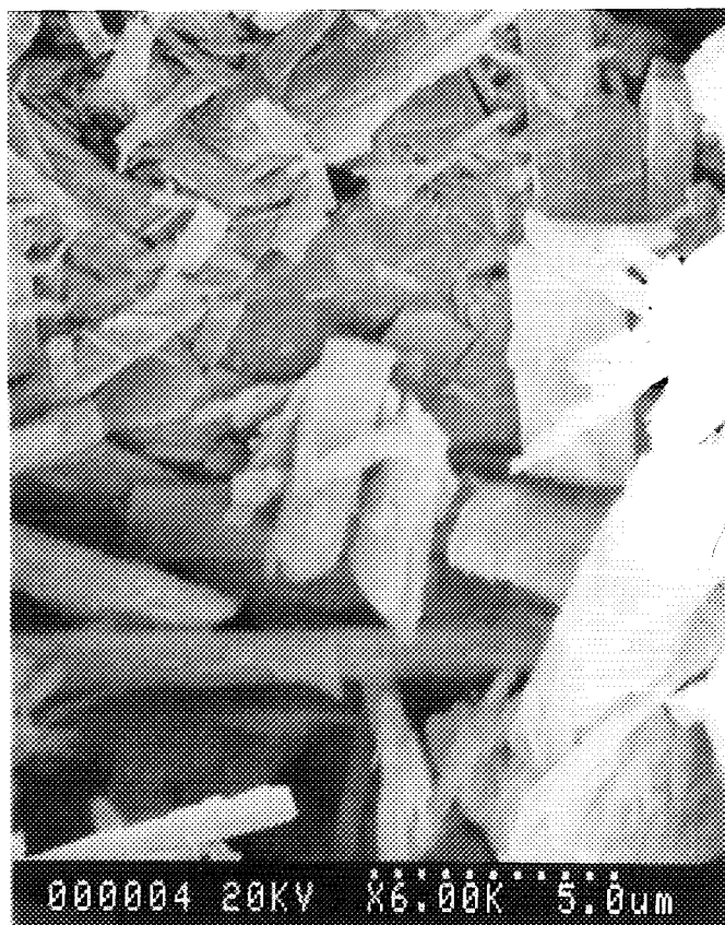
FIG. 4. Scanning electron micrograph of reactant \text{MoO}_3 .
